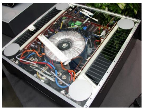
What accounts for this prowess? I was at a loss to explain it in the Trinity Preamp: I'm still at a loss now with the A1. Look at the photo of the interior of the chassis. An oversized, 1200 VA mains transformer takes up nearly 50% of the internal footprint and probably accounts for most its 90lbs. I'm sure it's a key part of the answer, but exactly how it factors in, I don't know.
